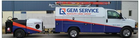
The hydro jetting machine sends water through clogged pipes and drains at 4,000 PSI.
