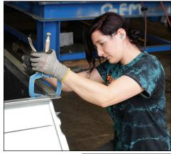
Above: GEM sheetmetal worker **Titania Adesi** assembles HVAC ducts and fittings at the GEM sheetmetal shop. Right: RLI operator **Molly Baumgartner** in her loader at First Solar's PGT-04 work site.
