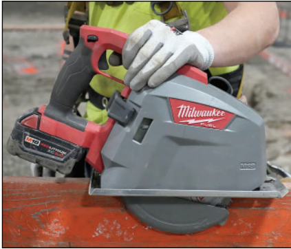
The 8-inch cordless saw reduces sparks and provides greater control of where the sparks will go.
