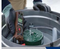
Motor amp reading is part of testing/balancing, ensuring that the motor is operating within the ratings, not over amping - and saving electrical costs for the owner.
